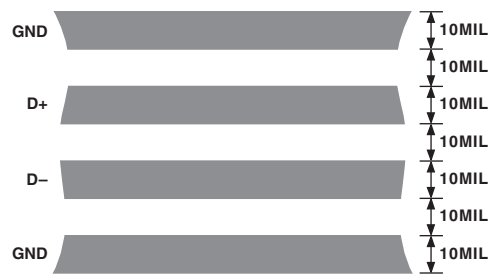
Figure 4. Arrangement of Signal Tracks
